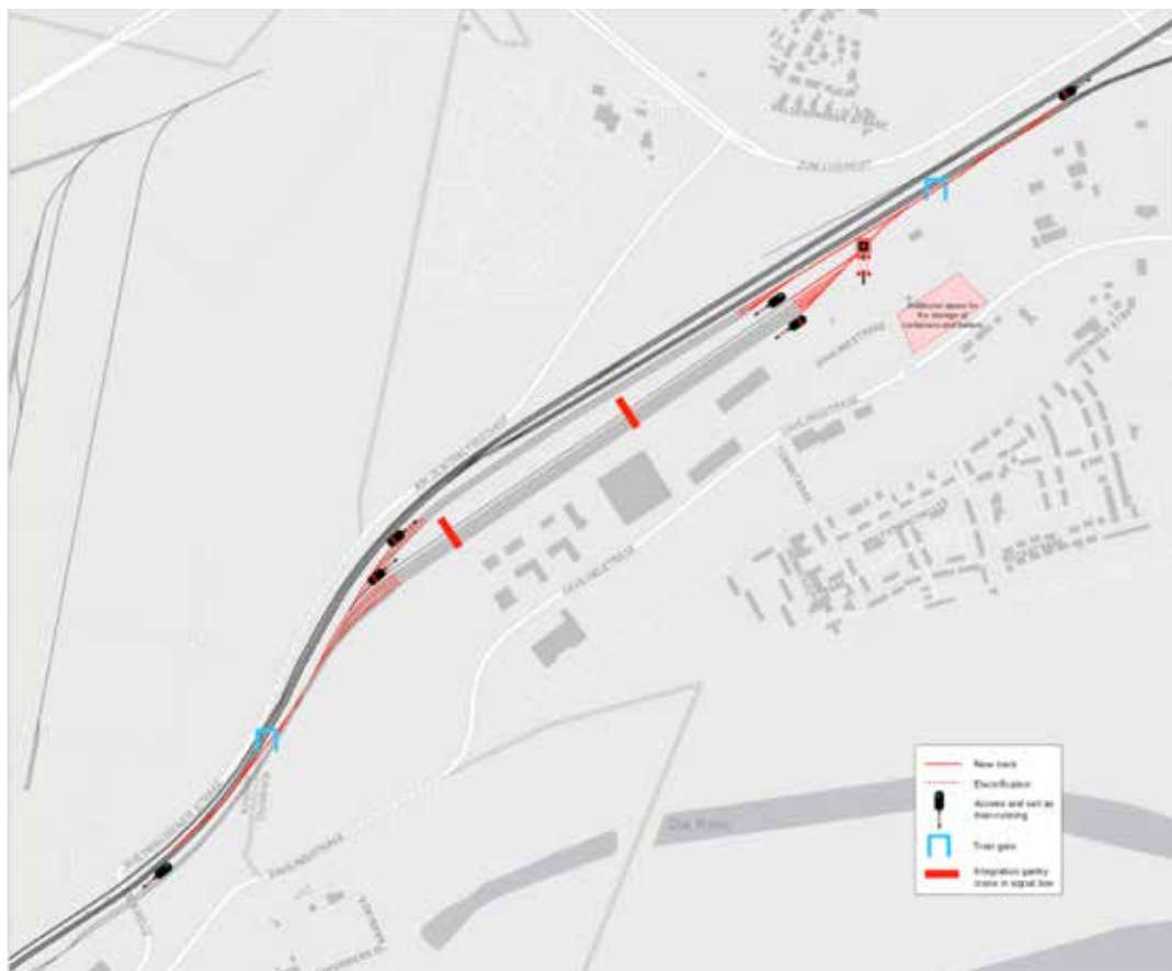
Figure 5.7 Duisburg-Hohenbudberg Logport III, infrastructural measures, option 2
