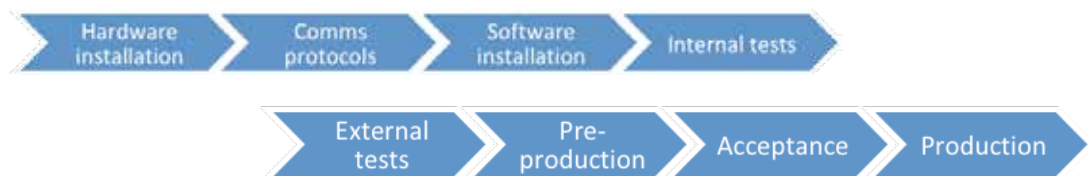
Figure 5.1 The sequence of steps for setting up the ERFLS telematics system at the terminals, from component installation to system commissioning
