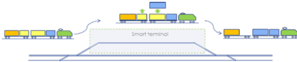
Figure 2.3 Ideally a smart terminal provides through sidings, and handling allows the main line locomotive to remain in the train composition
